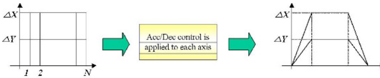
Fig. 4.2 Change to pulse profile after Acc/Dec control
